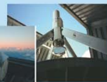
The stiff carbon fibre spider support of MITO telescope
