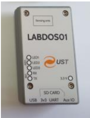
LABDOS spectrometer energy deposited in a Silicon diode by ionizing radiation
