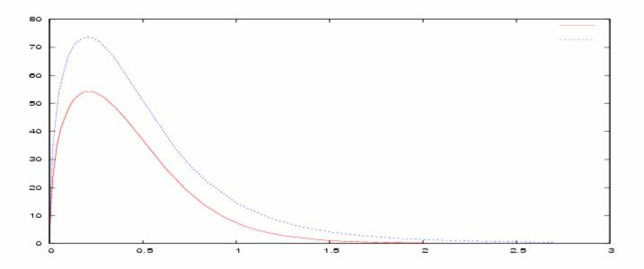
DM fluctuations today  $\overline{\Delta}(z=0,k)$  vs.  $k r_{lin}$ . Red= thermal FD initial. Blue =  $\chi$ -sterile neutrinos. Initial value  $\overline{\Delta}(k) = 1$ .
