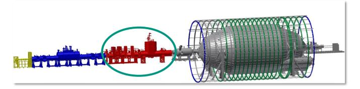
**Task:** Adiabatically guiding of beta electrons from source to spectrometer and elimination of tritium flow towards spectrometer
