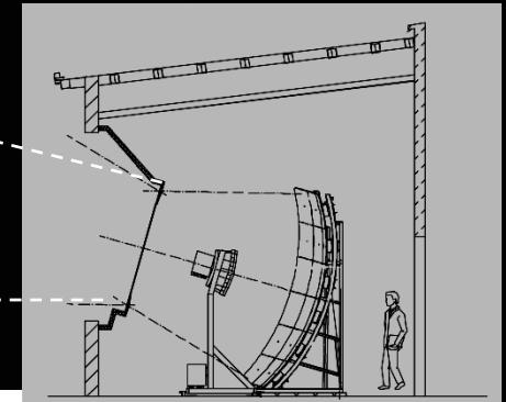
Fluorescence telescopes “see” the UV light emitted by  $N_2$  molecules excited by shower electrons
