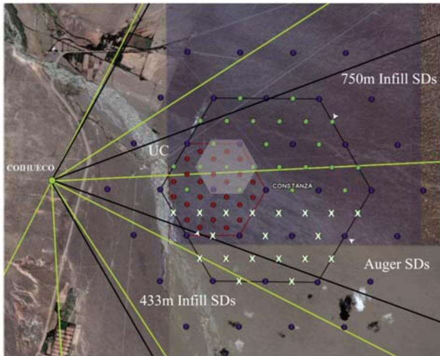
85 pairs of water-Cherenkov detector plus muon counter.
