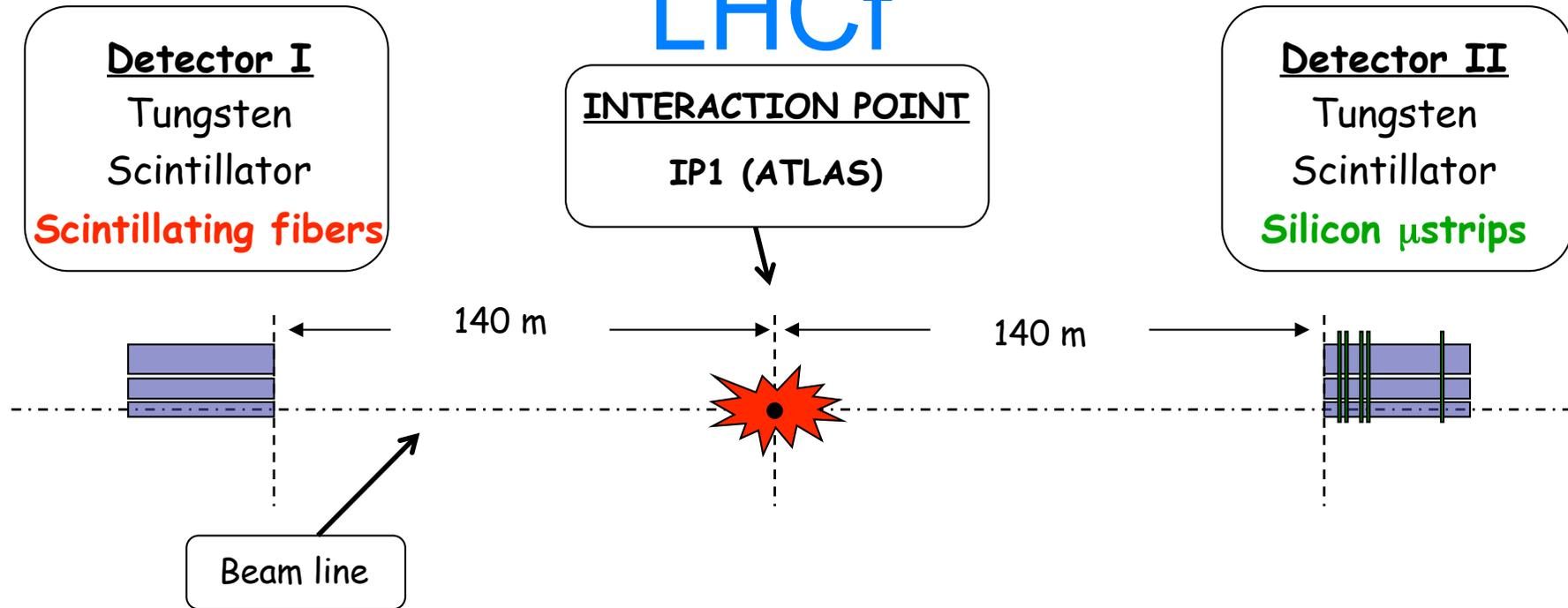
Detectors should measure energy and position of  $\gamma$  from  $\pi^0$  decays  $\longrightarrow$  e.m. calorimeters with position sensitive layers
