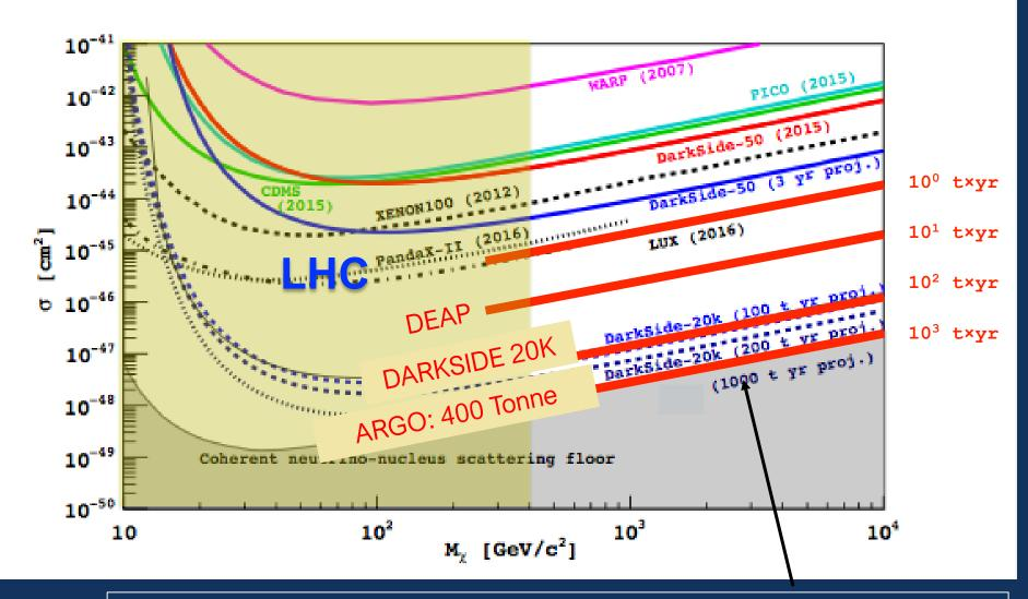
Future objective for the Global Argon Dark Matter Collaboration: A ~400 ton Liquid Argon detector with optimum technology and site. Excellent sensitivity and electron discrimination at the neutrino floor. Advantage over Xe: No interference from solar neutrinos for Dark Matter signals.
