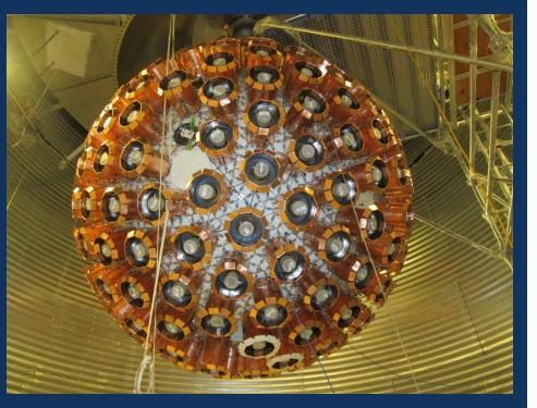
3.6 Tonnes of Liquid Argon: Dark Matter particles give very short bursts of light, gamma rays and electrons 200 times longer, enabling them to be separated.
