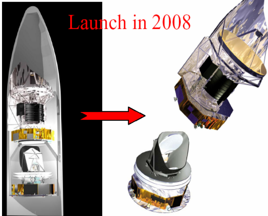
FIG 1.11.— Planck and Herschel ready for launch under the Ariane 5 fairing. The two satellites separate just after launch and proceed independently to their final orbits. View courtesy of Alcatel Space (Cannes).
