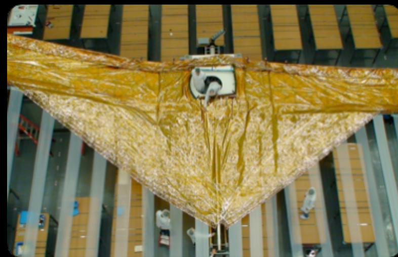
Sunshield deployment tests
