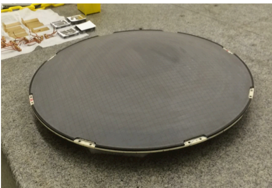
Thin, low loss, high thermal conductivity alumina filters and lenses with epoxy-based antireflection coating
